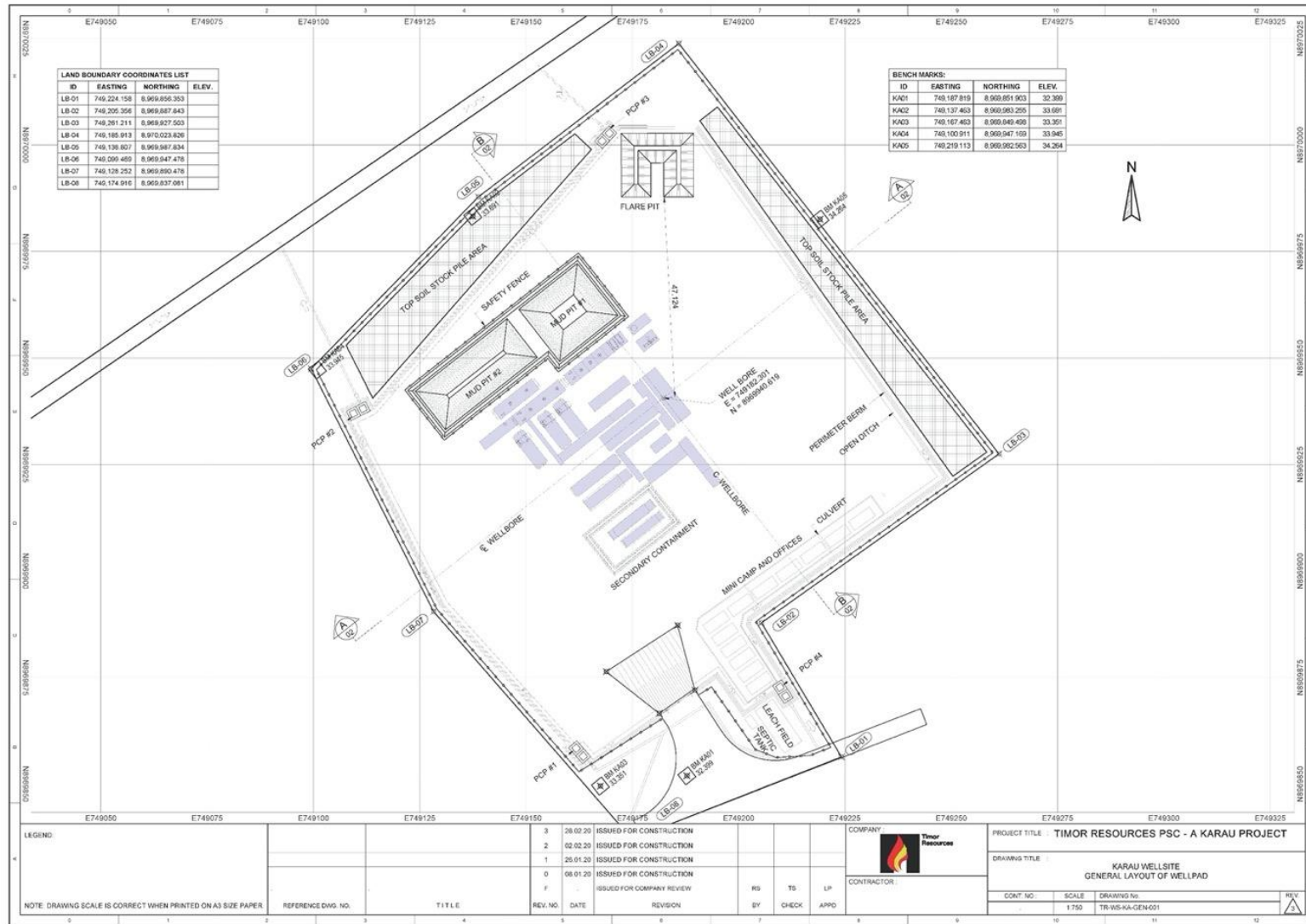
Figure 2 - Sample Site Plan (Karau-1) showing stockpile locations
