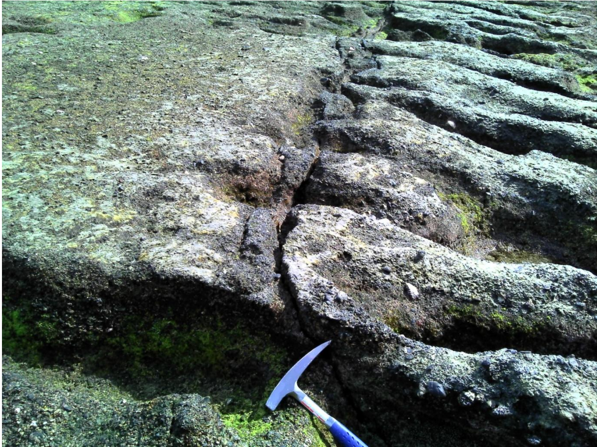
Plate 6-40 A geological fault is visible in the calcarenite running parallel to the beach
