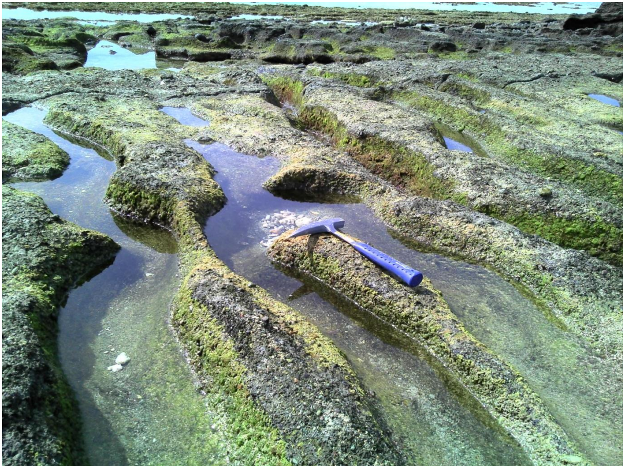
Plate 6-39 The calcarenite is characterised by dissolution channels across the surface
