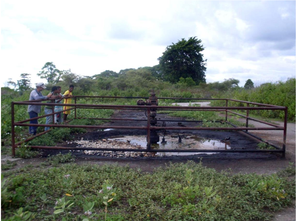
Plate 8-12 Example of contamination around a Suai oil bore
