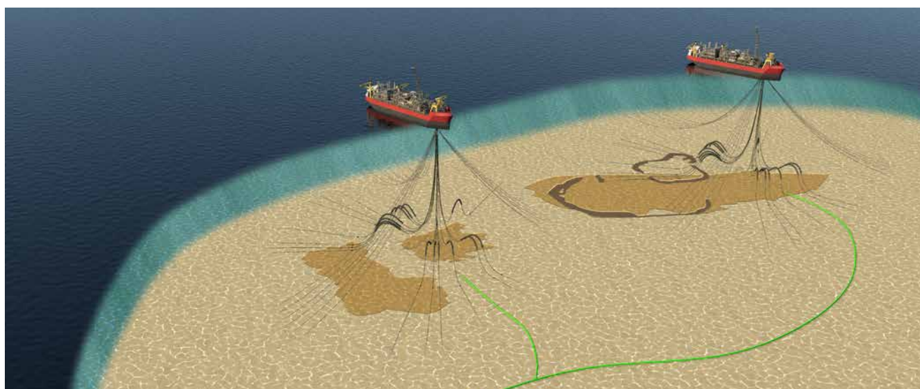
Browse FPSO development concept over the Brecknock, Calliance and Torosa fields (not to scale)
