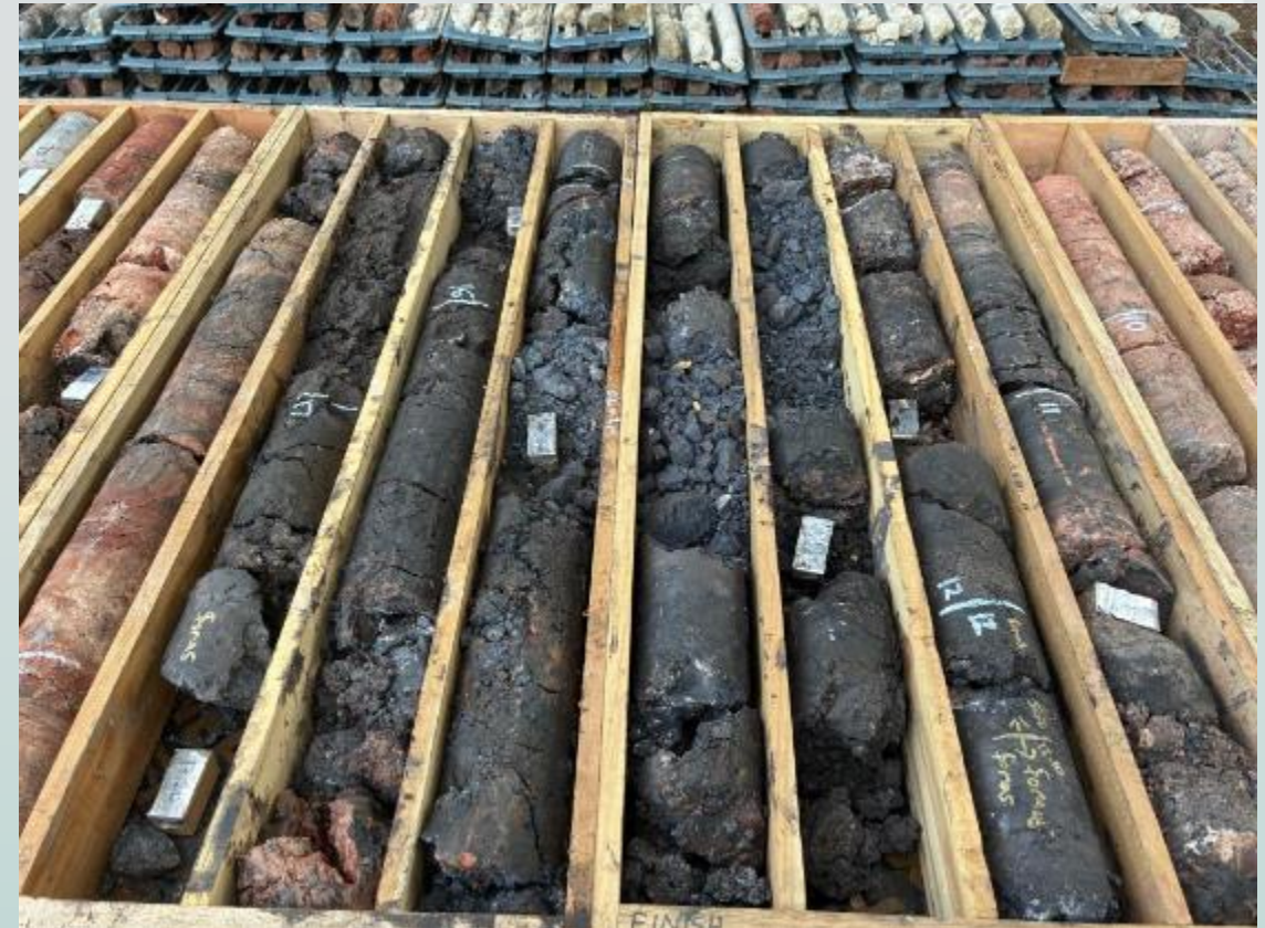
Core from EMDD040, including 2.5m assayed at 50.8% Mn. Refer to ASX announcement dated: 18 December 2025 "High Grade Ira Miri Mn Assays"
