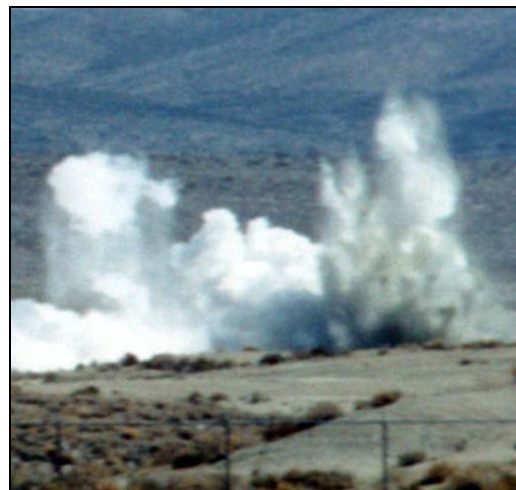
Figure 21. DOE's Burro experiments with LNG vapor dispersion, where Rapid Phase Transition shows explosive behavior. [41]
