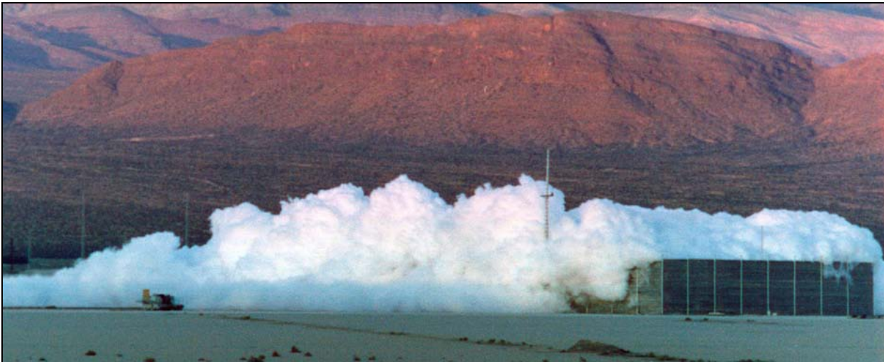
Figure 19. Experiments to contain a dispersing natural gas cloud with a physical barrier (Falcon LNG vapor barrier experiments, Nevada Test Site 1987, from [41]).
